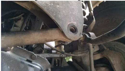
4. Locate the 1/4" hole below the bump stop plate. Using this hole as a guide, with a 1/4" drill bit, drill a hole opposite of this hole through the other side plate. Next drill both holes out to a size of a 1/2".
