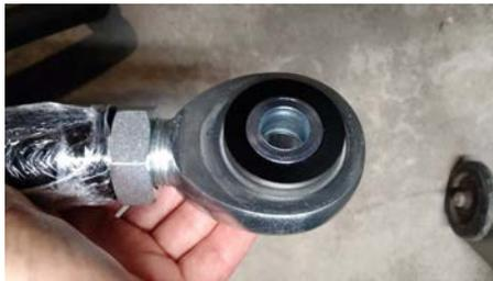
7. Install the right handed Heim joint and spacers into the trac-bar frame mount and insert the stock bolt. Tighten but don't torque the bolt yet. **Note: If you have a Fabtech frame mount you may need to clearance the mount to fit the Heim joint correctly.**
