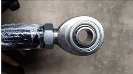
6. The right handed Heim joint goes on the frame side of the bar. Insert the Heim spacers into the Heim joint. Place the Delrin isolators over the Heim spacers with the angled side towards the ball.
