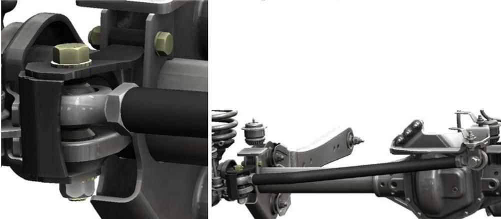
10. Using the same measurement locations as you did in step 1, measure the points again. Adjust the length of the bar by turning the bar right to shorten or left to lengthen, try to match your measurement in step one.
