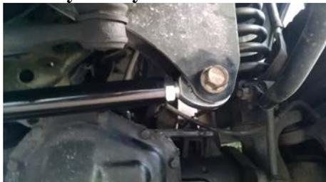
8. Insert the high-miss spacers into the left handed Hiem joint. Place the tapered spacer end into the axle mount hole.
