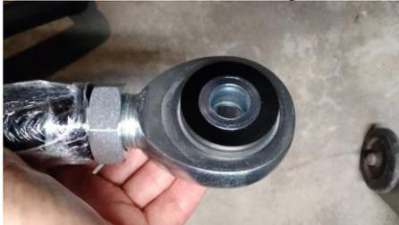
11. Install the Heim joint and spacers into the trac-bar frame mount and insert the stock bolt.
