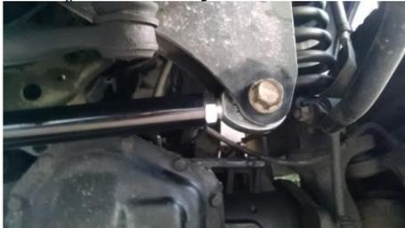
12. Using the same measurement locations as you did in step 1, measure the points again. Adjust the length of the bar by threading the heim joint in or out, to match your measurement in step one. **Note:** You will have to remove the bolt and heim joint from the frame mount in order to thread the heim in or out for adjustment.
