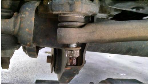
3. Remove the stock bolt and nut from the trac-bar frame mount, do not discard, they will be reused on the Trac-inator. Remove the stock trac-bar. **Note:** Tie-downs attached to the axle and frame may be necessary to prevent the axle from shifting after removing the bar, this will aid when installing the new bar.
