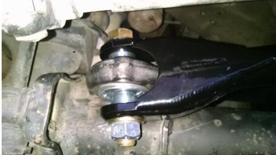
9. Thread the 1.25" Jam nut (BC-1059) onto the 1.25" Heim Joint (BC-1060) shaft. Then thread the 1.25" heim joint into the end of the Main bar, leaving approximately  $\frac{3}{16}$ " of thread exposed between the jam nut and heim joint.
