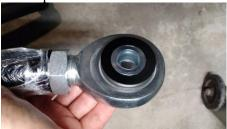
11. Install the Heim joint and spacers into the trac-bar frame mount and insert the provided M20 bolt with washers on either end. **Note:** If you have a Fabtech frame mount you may need to clearance the mount to fit the Heim joint correctly.
