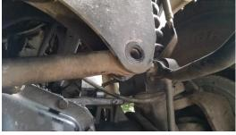
**4.** Using a Ball-joint press, remove the ball-joint from the axle mount. Depending on the type of press you use, you may have to cut off the threaded end of the ball-joint to fit the press over the ball-joint.
