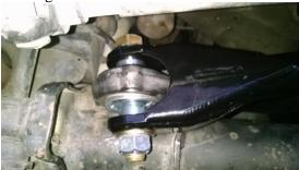
**9.** Thread the 1.25" Jam nut onto the 1.25" Heim Joint shaft. Then thread the 1.25" heim joint into the end of the Main bar, leaving approximately 3/16" of thread exposed between the jam nut and heim joint.
