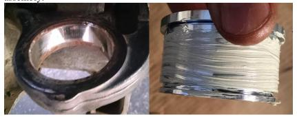
6. Place the Uniball cup assembly in the top side of the ball-joint hole. Make sure the Uniball cup assembly is concentric in the hole. Use a Ball-joint press to press it all the way down until the cup lip bottoms out. Be sure when using the ball joint press to only put force on the cup wall, NOT on the bearing in the center.
