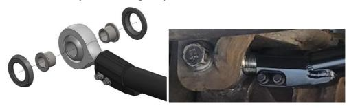
**8.** Install the uniball spacers into the uniball as shown, and install the assembly into the frame side track bar mount on the truck. Place the stock bolt into the mount and assembly, but do not tighten yet.
