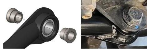
**9.** With the new bar in and bolts in place, recheck the position of the axle as you did in the first step. If you need to re-adjust the bar, do it now.
